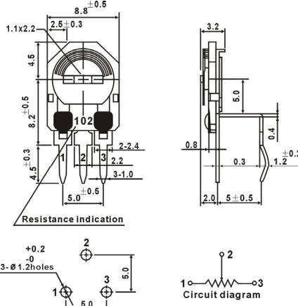
MOUNTING DETAIL TOLERANCE ±0.1
