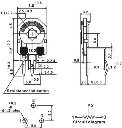
MOUNTING DETAIL TOLERANCE ±0.1
